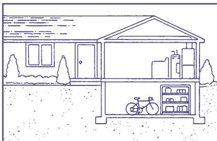
You should furnish areas that have been wet floodproofed with light, portable furniture that can be easily and quickly moved before a flood. Objects that are difficult to move, such as furnaces, water heaters, appliances, and bookcases, are either put on platforms or reinstalled upstairs.
