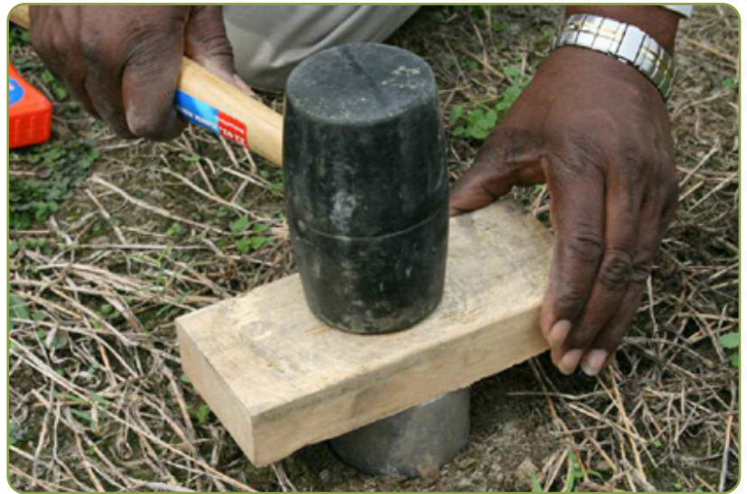
Simplified Method to Measure Bulk Density Photo: NRCS National Soil Survey Center
