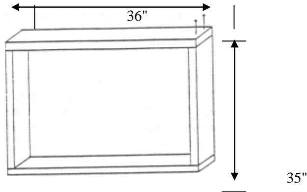
Mark the edges of each frame on both 9' long boards. Lay three of the frames aside.
