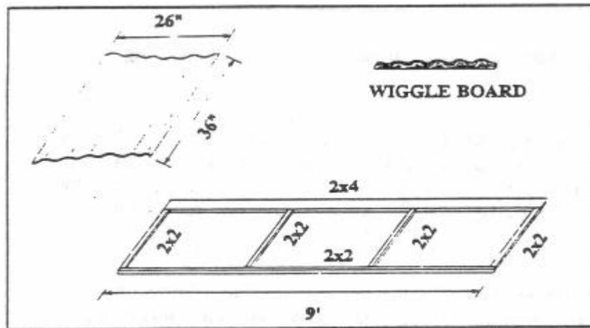
Lay the lid frame, brace side down, on the compartment frame with the 2x4 piece at the rear. Attach the two together with the butt hinges. Pilot drill the screw holes first to avoid splitting wood.
