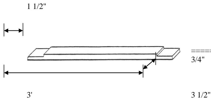
3. Make four lap jointed frames 3' square with the 16 boards. Connect each lap joint with carpenter's glue and four wood screws. Pilot drill the screw holes with a 1/8" bit first to prevent the board ends from splitting.
