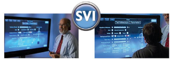
The Sanet Vision Integrator (SVI) Using a 50" touch screen monitor, the instrument is designed to improve visual abilities for a wide range of patients with learning problems, sports vision enhancement, amblyopia, and traumatic brain injury.
