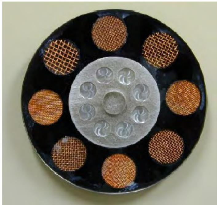
**Figure 9. Fluoroscopic test tool—view of embedded test objects.**
