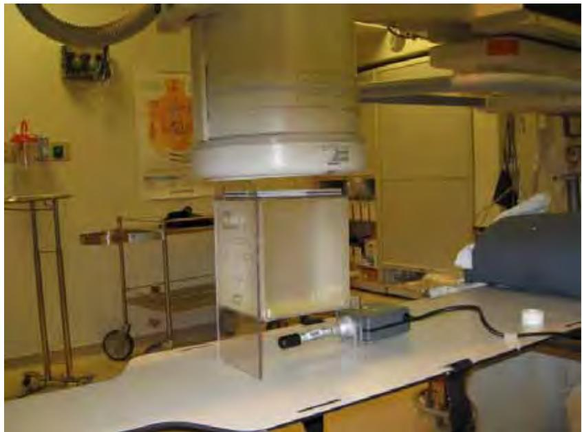
10. Place a couple pieces of tape on the table to locate the position of the phantom. This will assist you later when you need to remove the MDH and reposition the phantom for the image quality procedure.
