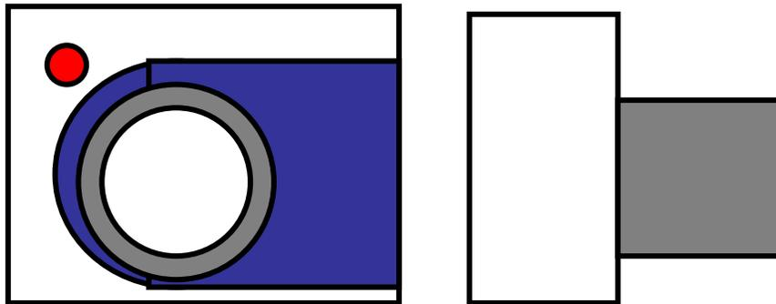
Figure B. Digital camera design hand-held x-ray unit. There can be some variation in cylinder aperture (cone) length. At least one of the manufacturers using the camera body design offers an optional back-scatter shield.
