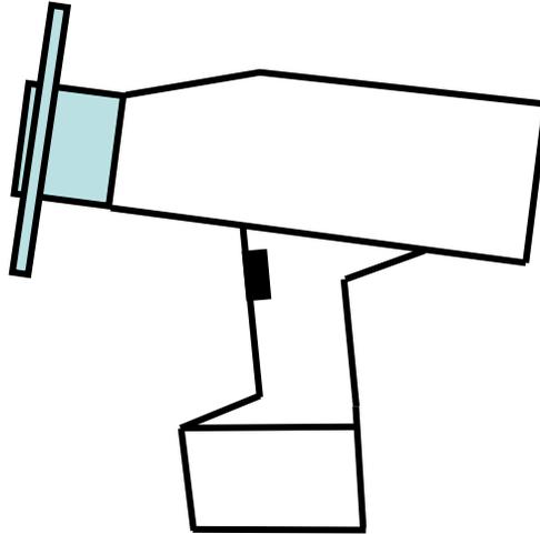
Figure A. Design similar to a cutie-pie meter with an integral back-scatter shield.
