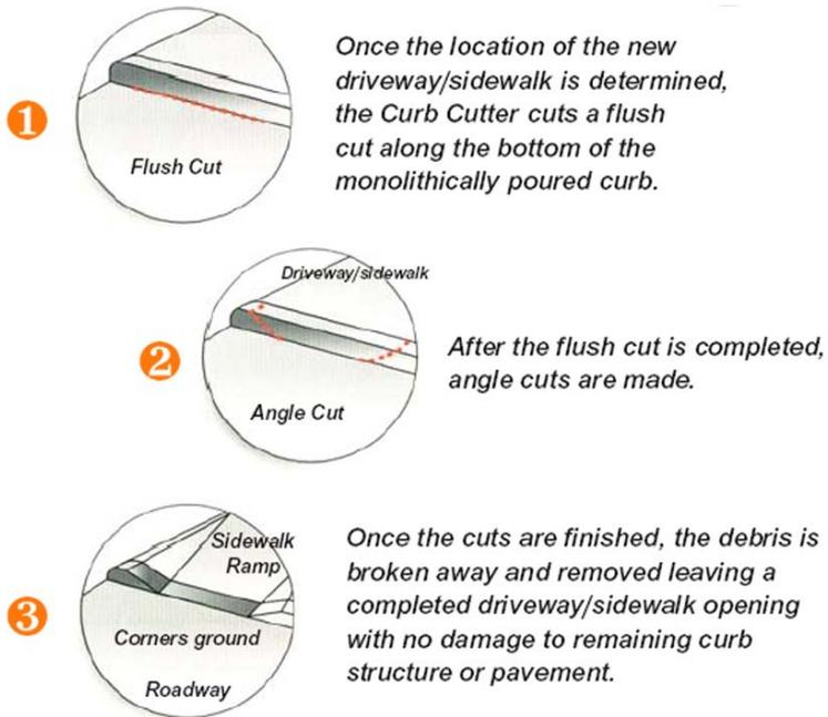
**How a curb cutting machine makes curbs.**
