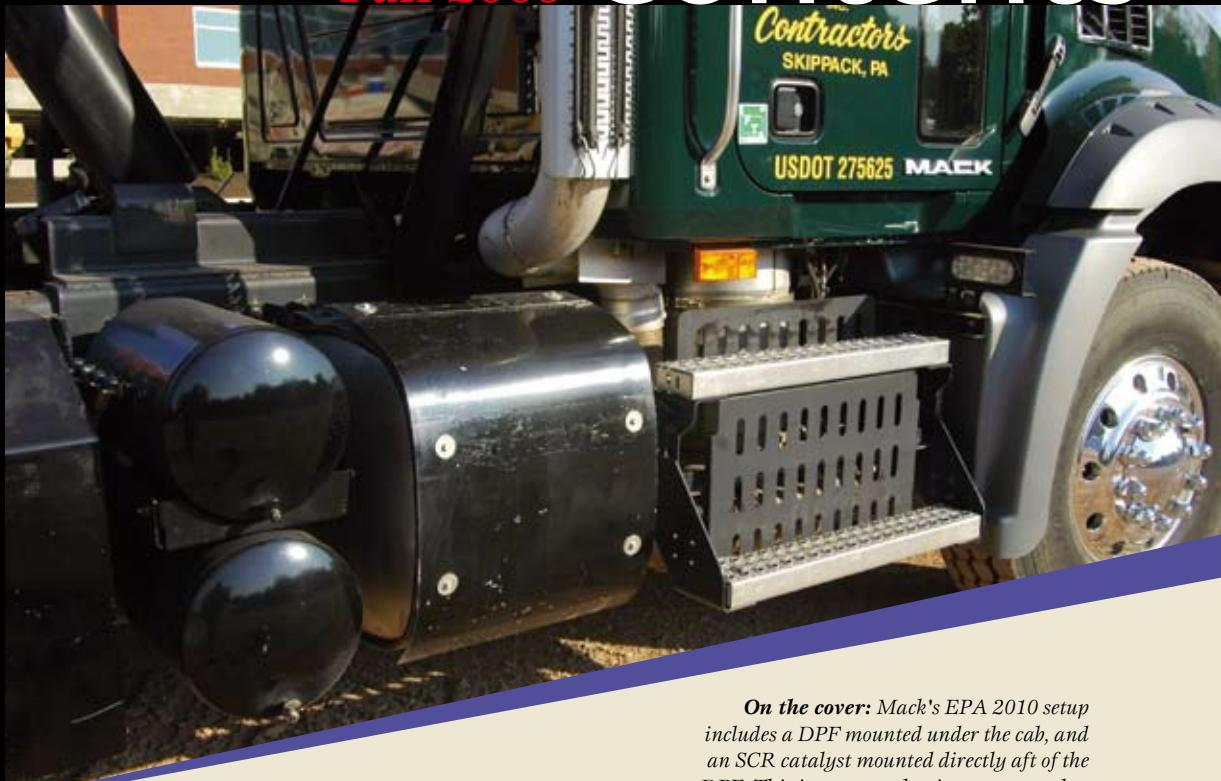
**On the cover:** Mack's EPA 2010 setup includes a DPF mounted under the cab, and an SCR catalyst mounted directly aft of the DPF. This is a pre-production prototype, but Mack says the look hasn't changed.
