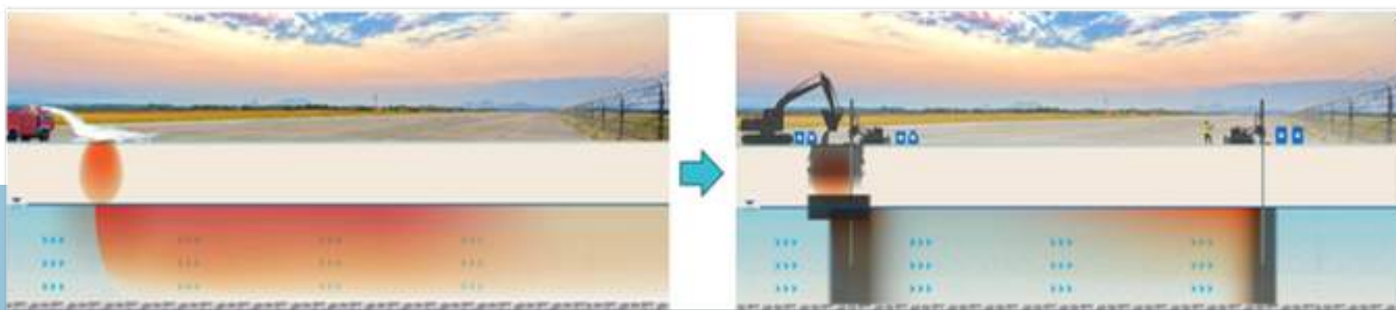
Figure 2: In the left image, aqueous film-forming foam (AFFF) containing PFAS is sprayed on an airport runway, causing a PFAS plume to develop in groundwater. In the right image, CAC is applied beneath the source area and in a downgradient permeable barrier as PER measures to mitigate PFAS exposure risk. Image source - REGENESIS.
