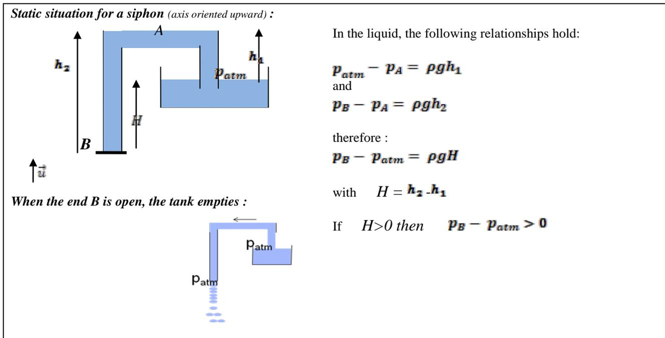
Figure 1. In a static situation, the pressure exerted on the object closing the lower end of the tube is larger than the atmospheric pressure.
