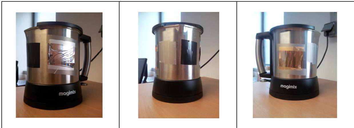
Measures of the respective emitted powers, indicated with equivalent temperature (IR thermometer) when the water in the boiler is boiling:
