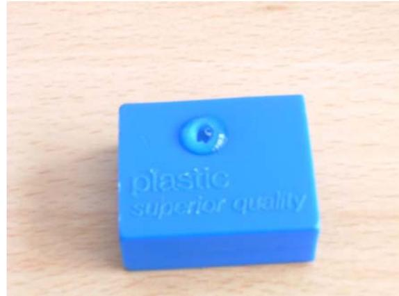
Fig. 3. Water kept outside a „pore“ due to its surface tension
