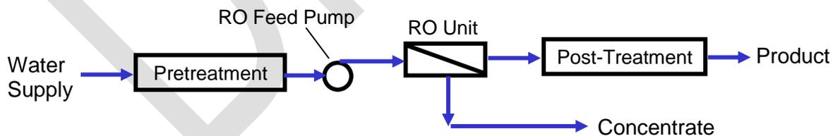
Figure 1 - Basic components of a RO desalination process
