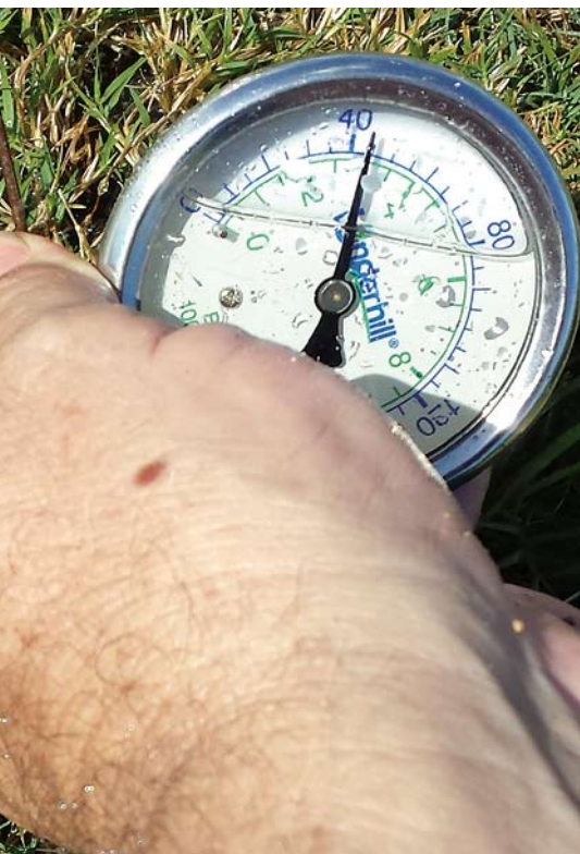
Fig. 7 After sprinkler head nozzles in the football field were downsized, the pressure and uniformity increased because there was less friction loss in pipes and there was much better coverage in all areas including the perimeter areas nearest the track.
