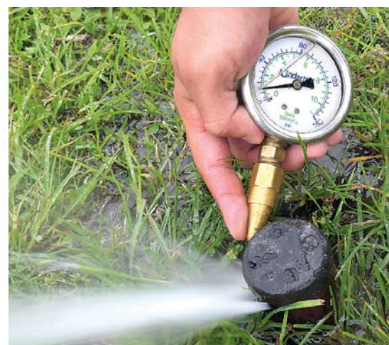
Fig. 3 The soccer field sprinkler heads had only 15 psi pressure in the nozzles when the irrigation zone was running. Pressure was measured with a pressure gauge and a pitot tube in the nozzle. This "dynamic" pressure was too small. Ignore "static" pressure when the irrigation system is not running. If you observe pressure anywhere else, such as the pump, realize that it won't tell you about the ability of the irrigation system to cover an area.
