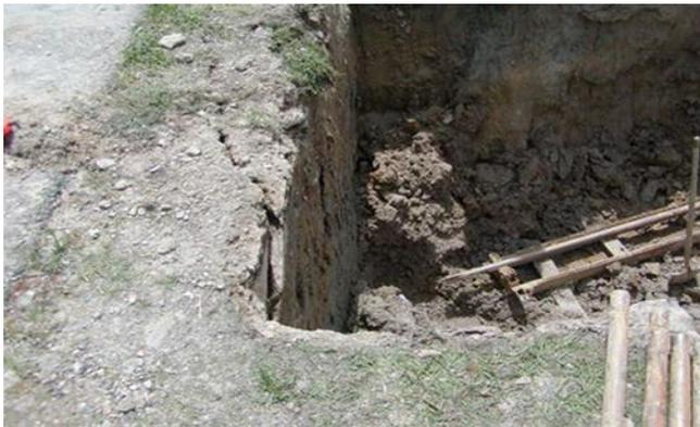
The ground surface on the road side of the trench begins to fissure. Time: 1:05:50 PM.
