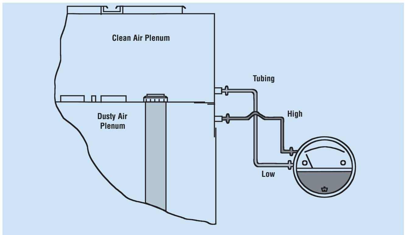
filter utilizes reverse air cleaning, the scale on the gauge should have zero in the center so that the differential pressures to the left of zero can be monitored during periods of reverse air flow cleaning.
