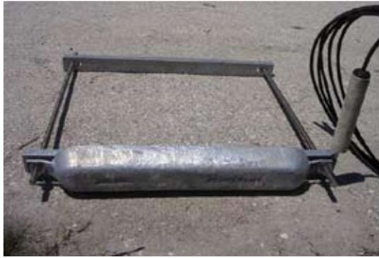
*Fig. 5: Bulk zinc anodes used to protect concrete piles in seawater*
