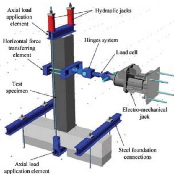
Fig. 4: Test setup
