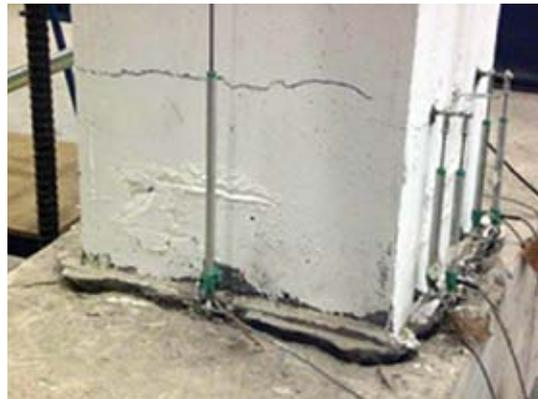
Fig. 11: Slip between jacket and foundation base
