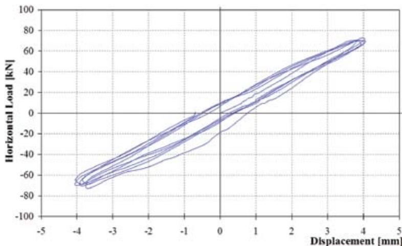
Fig. 7: Horizontal load versus displacement for the design load level. (Note: 1 mm = 0.039 in.; 1 kN = 225 lbf)
