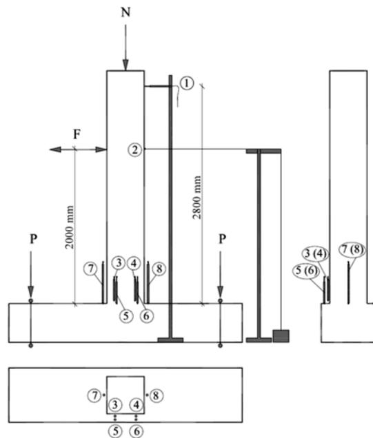
Fig. 6: Displacement measurement setup. (Note: 1 mm = 0.039 in.)
