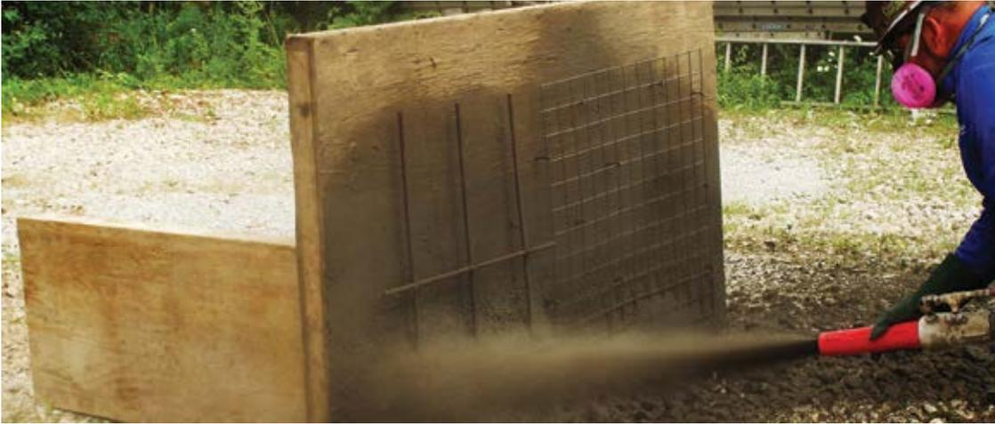
Fig. 5: Preparation of a shotcrete test panel
