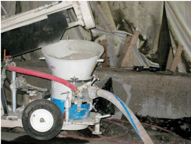
Fig 3: Dry-mix process rotary-bowl type shotcrete machine
