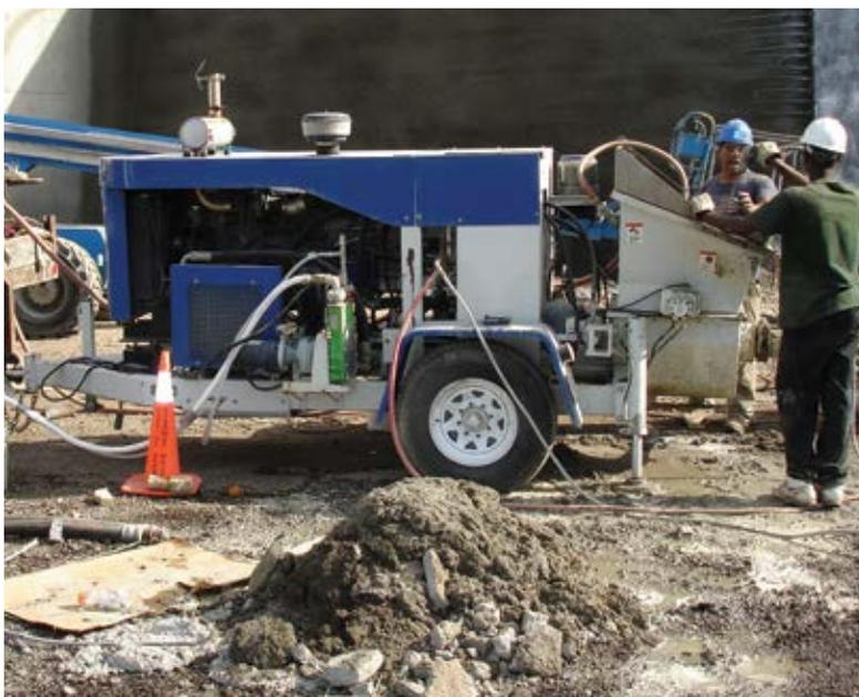
Fig. 4: Wet-mix shotcrete pump
