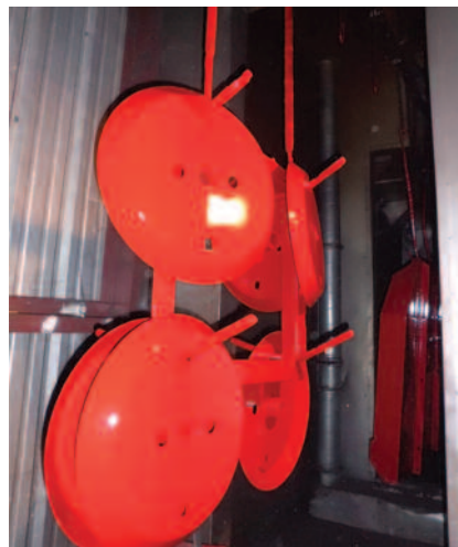
Both small and large parts are shown entering the curing oven.
