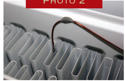
A thermocouple attached to a part using high-temperature epoxy resin. Note that the tail is also attached to the part to ensure there is no load on the thermocouple head.
