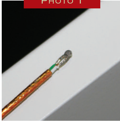
A typical pin head thermocouple.
