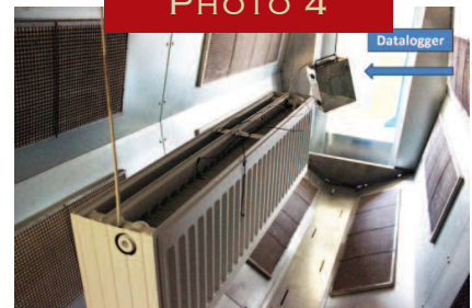
A part with thermocouples attached to the part and data logger is shown progressing through the oven.
