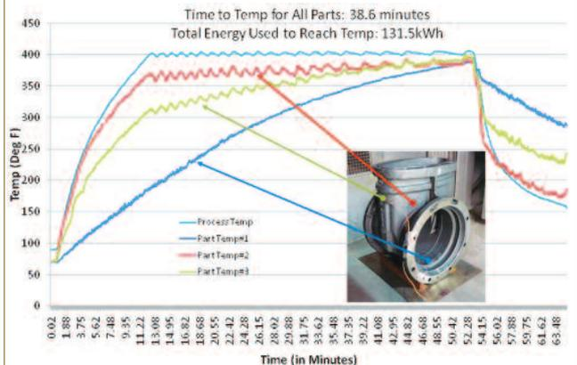
the use of 300kW of a combination of IR (127kW) and convection (173kW). In this test, the part reached temperature in 38.6 minutes while using 131.5kWh (shown in Figure 7 and Figure 8).
