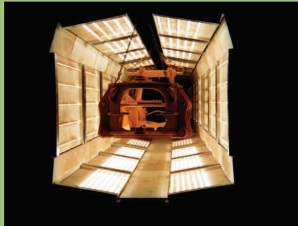
*An off-road vehicle frame is shown inside a combination oven. Photo courtesy of BGK Finishing Systems, Infrared Curing Solutions.*
