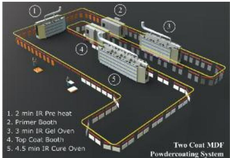
IR ovens are constructed, with a fully reflected concept, for multiple zone control. The key to curing the MDF parts is to direct the IR energy toward the edges of the board to drive the powder to a gel and then to the cure point along these difficult-to-heat areas. As a result, the edges seal quickly, preventing out-gassing.
