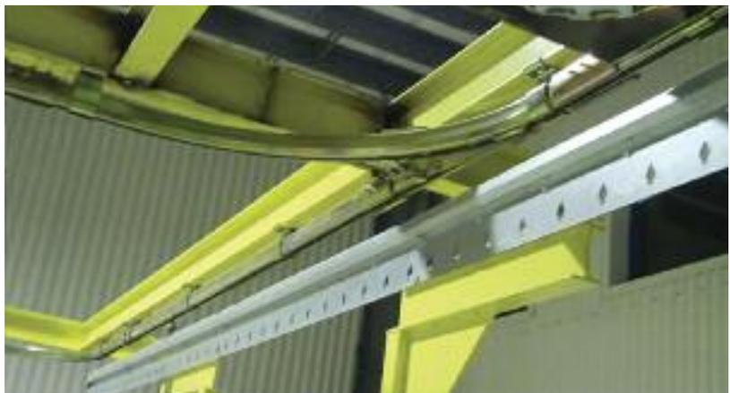
been installed to address those concerns mentioned previously. These lines are powered with gas catalytic IR ovens and a novel approach to conveying parts through the lines. The main advantages of these lines over traditional lines are lower capital investment, a smaller plant footprint, long-part capability (Figure 1), lower utility costs, and increased production throughput. The lines also achieve all the lean goals and drive manufacturing costs down.
