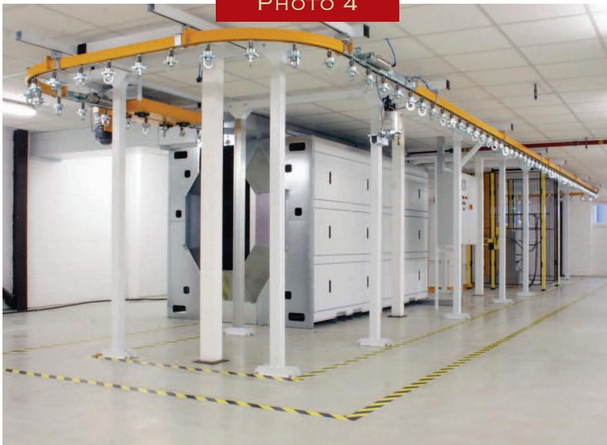
*This relatively small, two-section gas catalytic IR oven is suitable for handling a high mix of varied but relatively small components.*
