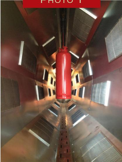
*The refurbishment line's oven design has been optimized to suit the complete range of LPG cylinder sizes.*
