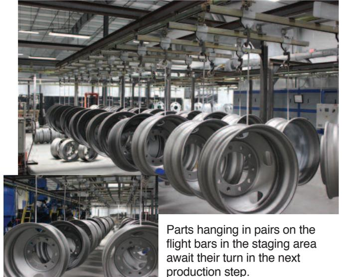
Parts hanging in pairs on the flight bars in the staging area await their turn in the next production step.
