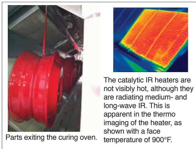
Parts exiting the curing oven.
