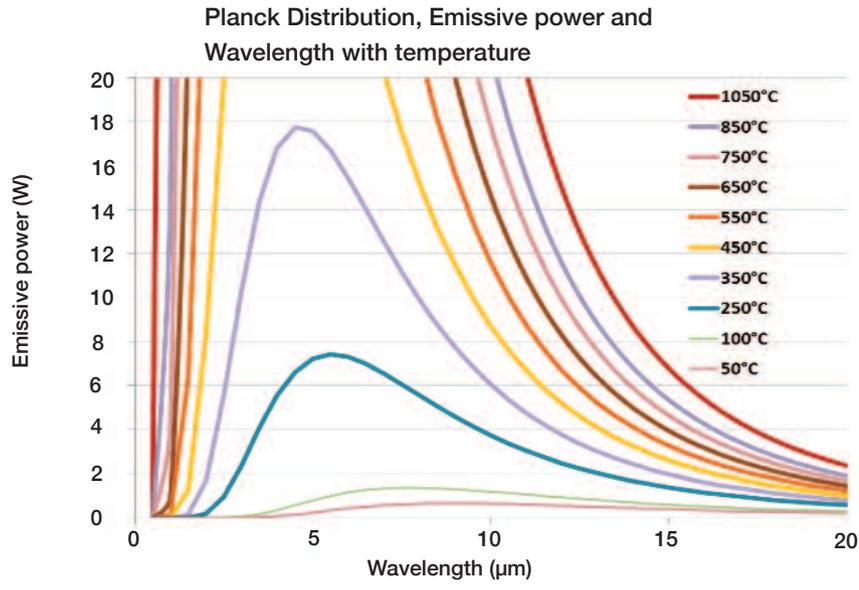
As the temperature decreases, the energy levels also drop, and the peak energy wavelength shifts to the longer wavelengths. The lowest temperatures from the 250°C, 100°C, and 50°C curves cannot be seen in the graph. When the graph is enlarged to see the lower temperature curves, this shift to the longer wavelengths is more apparent. However, the power intensity drops significantly.
