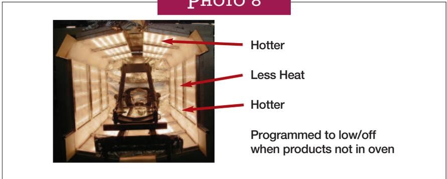
*PLC controls can be used to regulate temperatures in each zone*
