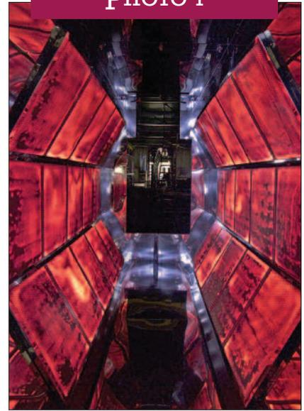
*Gas catalytic IR oven***PHOTO 2**
