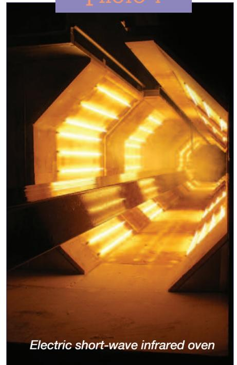
Electric short-wave infrared oven
