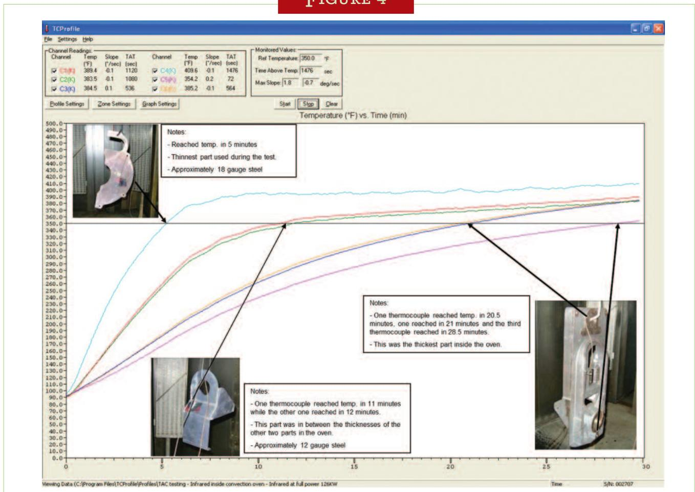
Temperature profiles of various size geometric parts with and without IR
