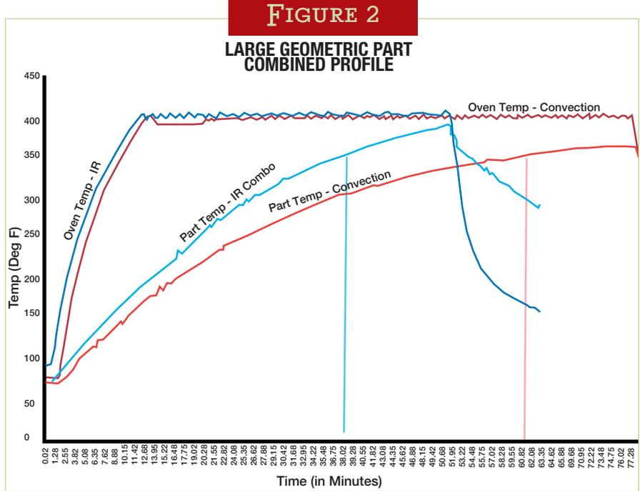
*Temperature profiles of large geometric part with and without IR*
