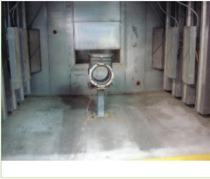
*Large geometric part with IR inside a batch convection oven*
