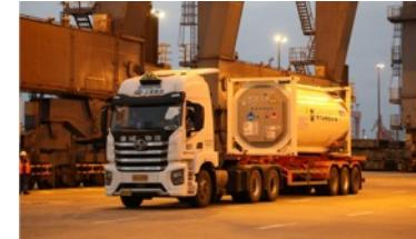
On November 18<sup>th</sup>, the world's first large-scale solid-state hydrogen storage device was shipped from Waigaoqiao Phase IV Dock. The magnesium-based storage tank uses a chemical reaction between hydrogen and magnesium alloy to store hydrogen in solid form. It offers high storage density, enhanced safety, and cost-effective convenience, facilitating long-distance, large-scale hydrogen transportation.
