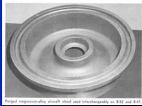
Forged magnesium alloy aircraft wheel used interchangeably on B-52 and B-47.
