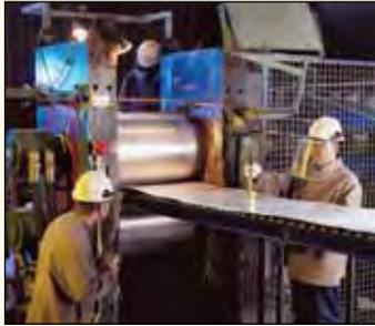
CSIRO's production-scale casting machine is a more time and cost efficient way to produce magnesium sheet. © Photo courtesy of CSIRO Australia. Used with permission.
