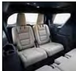
The Explorer (left) uses lightweight magnesium third-row seats (right) in both manual and power versions. © Photos courtesy of Ford Motor Company. Used with permission.
