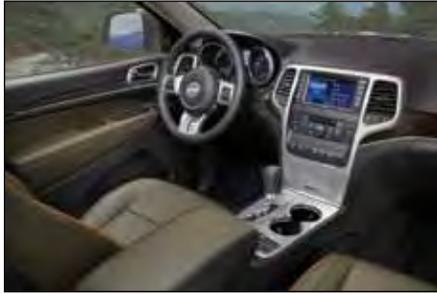
The Grand Cherokee's magnesium instrument panel has improved durability and lighter weight, connecting to navigation, safety and audio systems. © Photo courtesy of Chrysler Group, LLC. Used with permission.
