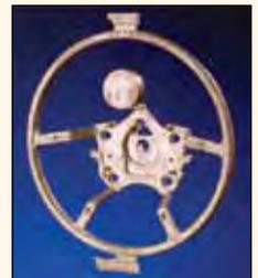
The ATM die casting process for this magnesium steering wheel armature uses a revolutionary feed system that is well-suited to magnesium. © Photo courtesy of CSIRO Australia. Used with permission.
