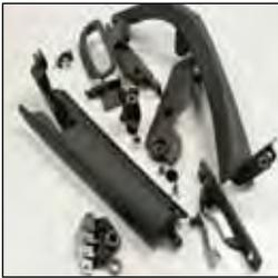
Ultra-light magnesium fixed roof components provide unyielding stiffness without affecting the Z06's low center of gravity. © Photo courtesy of Thixomat. Used with permission.
