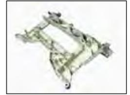
The AE44 magnesium engine cradle is the industry's first magnesium high-pressure die cast chassis component. © Photo courtesy of Meridian Lightweight Technologies Inc. Used with permission.
