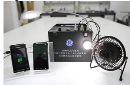
By optimizing structure and process for cathode air diffusion electrode and based on developing high performance oxygen reduction catalyst from manganese oxide, Power Lithium Battery Engineering Laboratory, Ningbo Institute of Material Technology, Chinese Academy of Sciences, develops successfully 1000Wh magnesium air battery.
