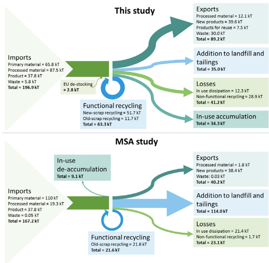
The bottom-up approach applied to developing the material flow analysis, i.e. quantifying each flow per application of Mg individually and then summing them together to get the values presented in Figure 1, meant that we could also determine how much Mg is used in which applications the EU.
