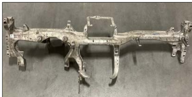
Figure 5: Cross car beam made of AM50 magnesium alloy. (Source: Meridian Lightweight Technologies.)
