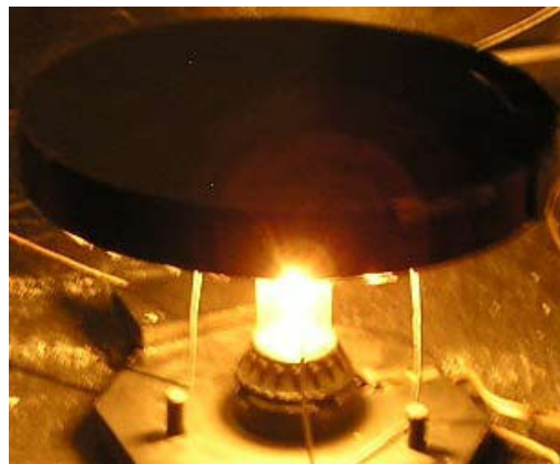
A wire stand can be fashioned to support the shade/cover over the tubular light.
