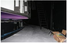
Space between dome spring-line and lighting valence is about 7" [17.78 cm]. This allows enough space for projector image output on the dome.
