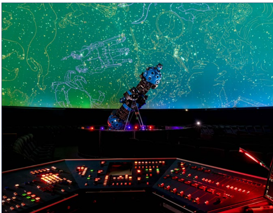
Picture 2: The Albert Einstein Spacearium/Sky Theater/Planetarium's Zeiss Model V1a star projector after both the dome had been replaced and the control console had been redesigned and been replaced following switching from Gyrosystems to Sky-Skan's S.P.I.C.E. automation. The original left and center panels had been dominated by the original controls for the Zeiss, while the right one was set up for the manual and automatic control of the theater's special effects and lighting via Gyrosystems. After much discussion and evaluating ergonomic ideas for the new layout, we and Sky-Skan came up with the functional design you see here. Again, the Zeiss controls—simplified but just as functional—were to the left and center, while all special effects are to the right along with the PC screen for the newer control system. And, as before with the original Gyrosystems automation, everything in the theater was still completely automated; still the first such planetarium in the world. This workhorse projector was retired in 2019 after serving daily for 40 years and was no longer able to be serviced by Zeiss. It now resides along with this control console at the sprawling NASM annex, the Steven F. Udvar-Hazy Center, at Dulles International Airport. The only other Zeiss V1a I know about was the one built for the planetarium in the Hong Kong Space Museum, which was also automated by Gyrosystems. (Source: Mark Avino, NASM)
