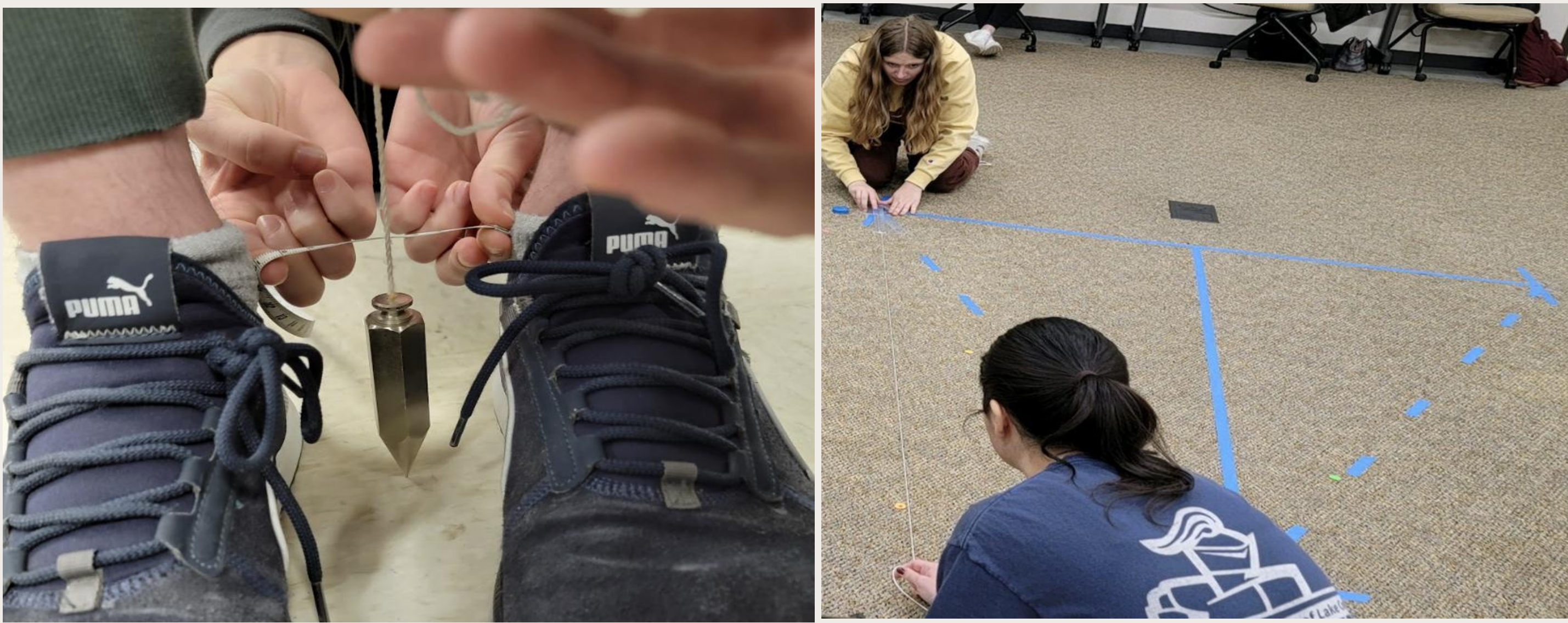
Figure 2. Measuring angular rotation error and end point error.
