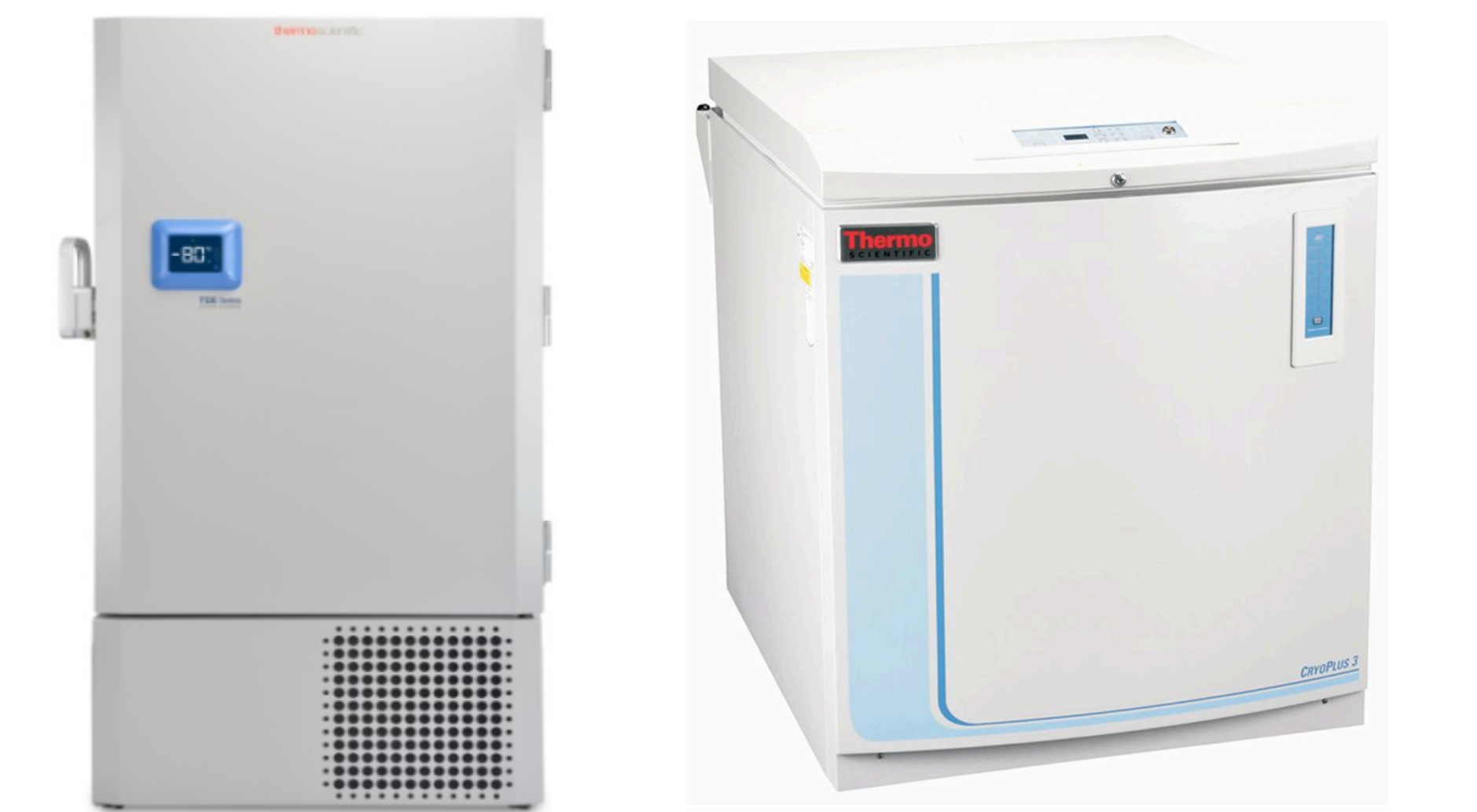
Figure 2. Thermo Scientific™ Ultra Low TSX Freezers with hydrocarbon refrigeration system, designed for high reliability and long-term sample storage and Cryomed controlled rate freezers designed to control the rate at which samples are frozen and to usher samples through the latent heat of fusion given off by samples during the freezing process. Both supporting criteria to help the biobank achieve order winners on for example performance, reliability and durability.
