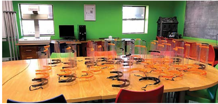
Rapid prototyping 3D Visors to address PPE shortages
