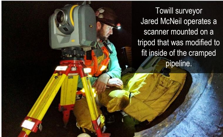
Towill surveyor Jared McNeil operates a scanner mounted on a tripod that was modified to fit inside of the cramped pipeline.
