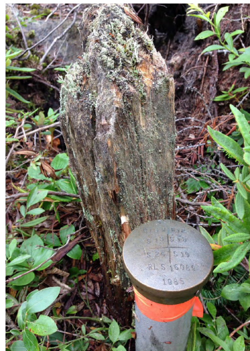
Brass-capped aluminum pipe monument (front) compared to previous wood post monument (back).
