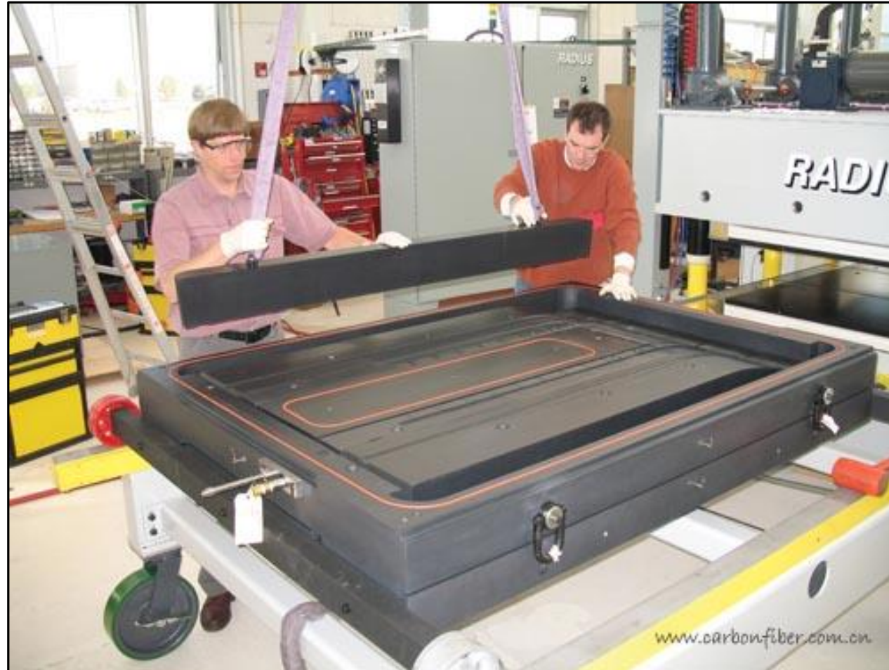
All black-anodized aluminum tooling
