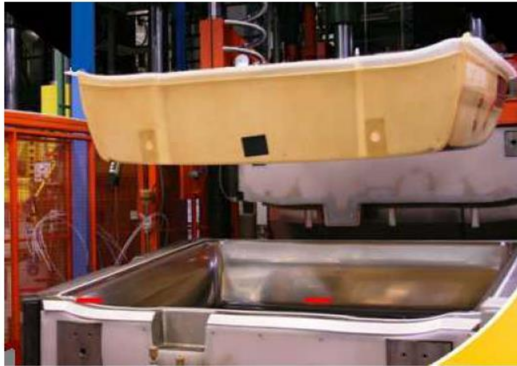
RTM mold and truck roof while demolding, source: Fritzmeier Composite
