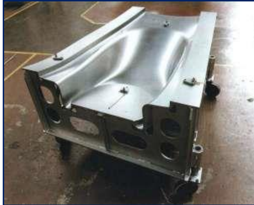
Steel Tool face cut from single billet
