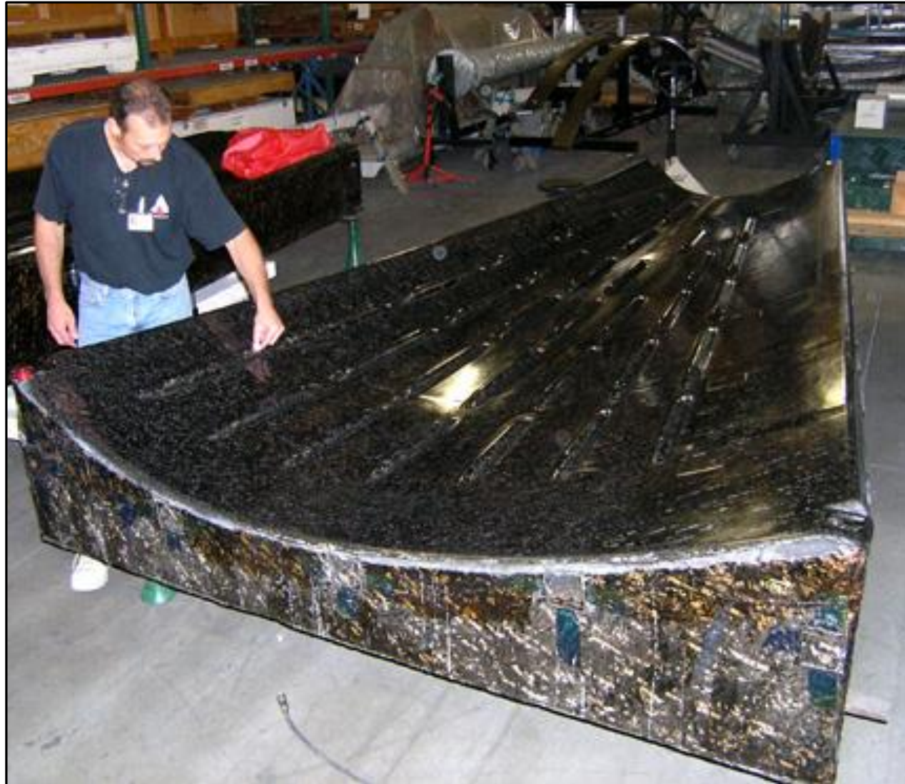
Internal Mold Line (IML) Beaded Stringer tool
