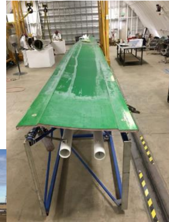
Portion of 60m spar cap infusion mold Courtesy DowAksa
