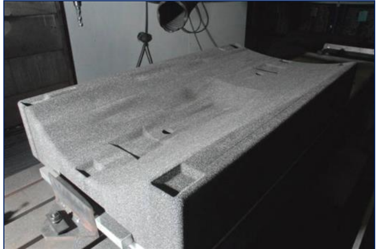
Finish-cut offset surface prior to prepreg
