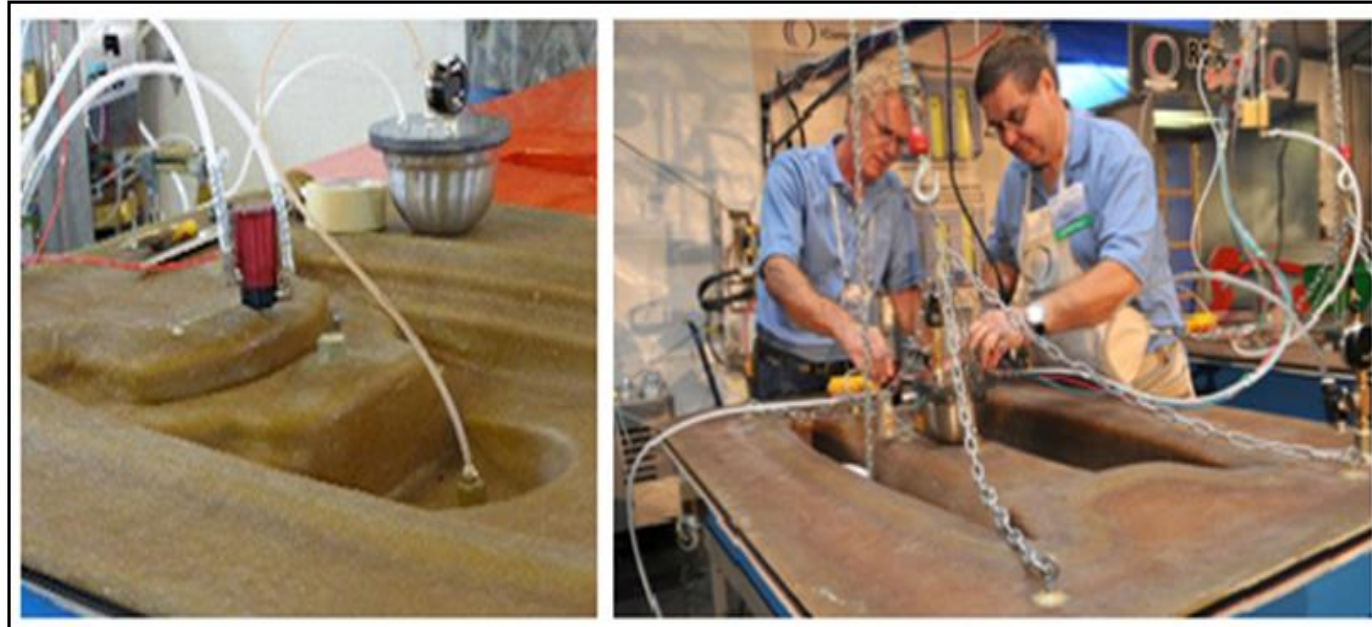
Example of LRTM process and vac/resin plumbing requirements
