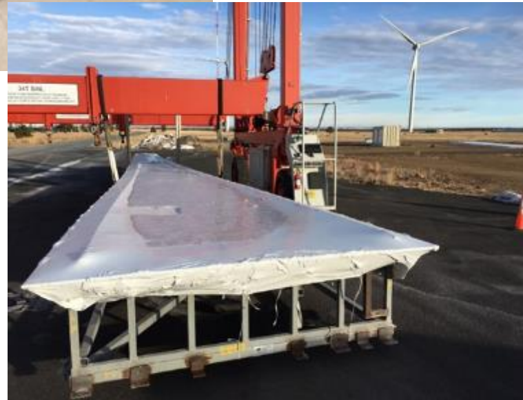
Large shear web mold Courtesy GE
