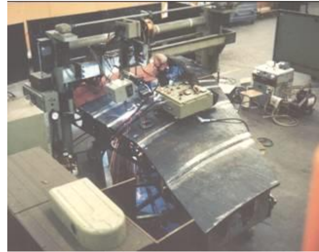
Welding Faceplate Sections
