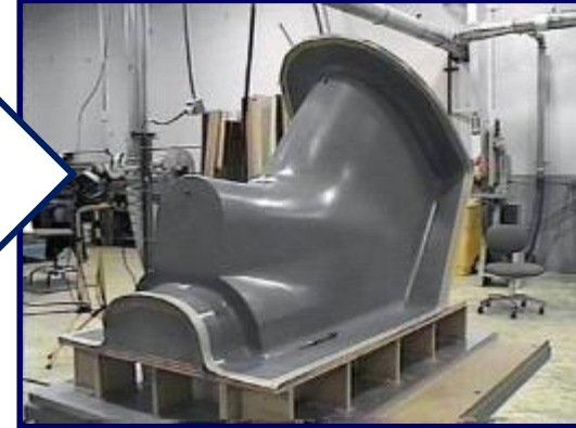
Machined Master Model
