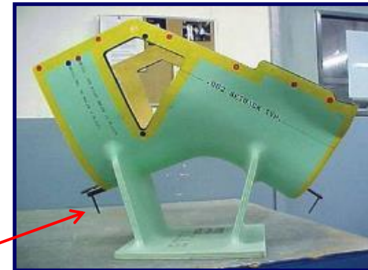
Trim & Drill Fixture (TDF) from MM
