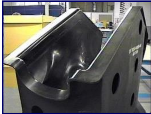
CFRP Layup Mold from MM
