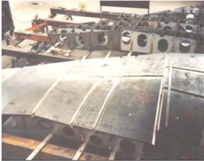
Steel Plates and Eggcrate Substructure
