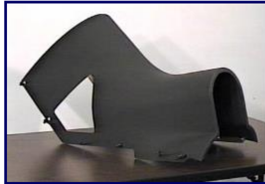
Final Kevlar/Epoxy Part made from the Layup Mold
