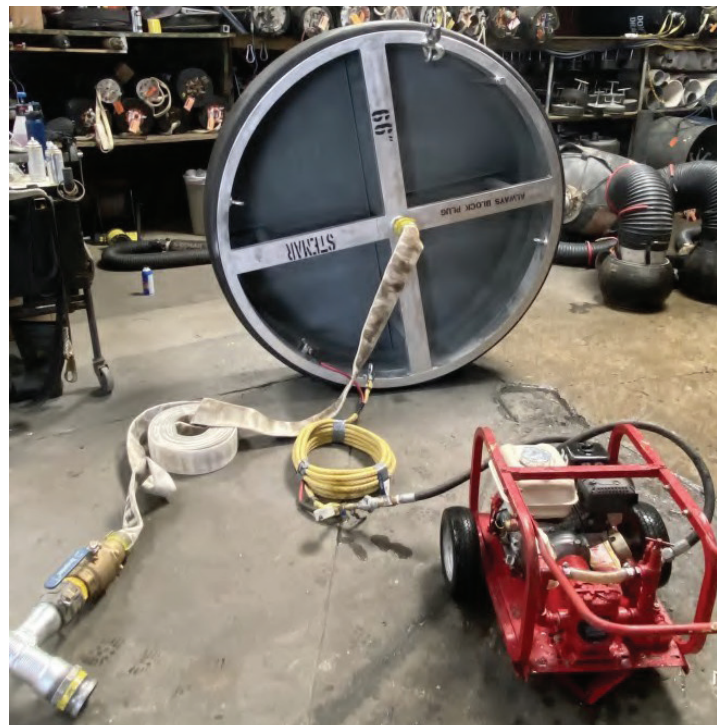
66" high-pressure test plug set up for fill via water pump (not pictured) and inflation and test via hydro-pump
