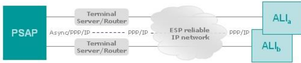
Figure 13 - PPP/IP network configuration
