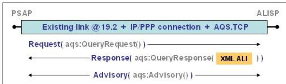
Figure 16 - Managed AQS binding (TCP version) illustration
