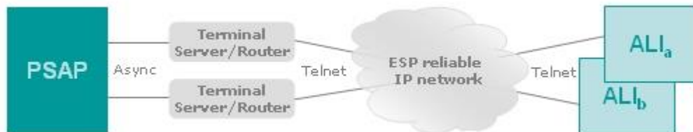
Figure 12 - IP backhaul network configuration
