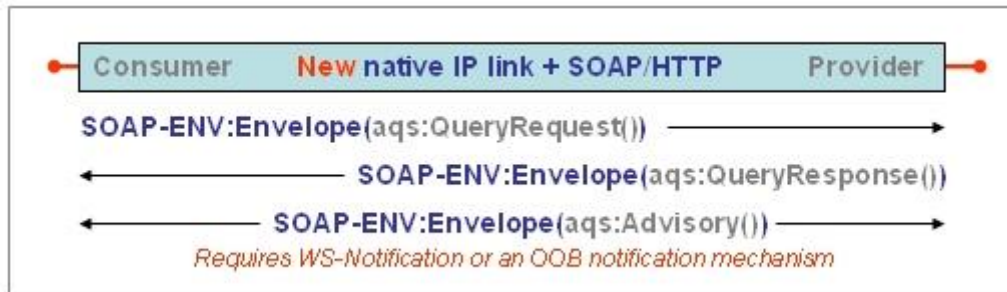
Figure 17 - Direct web services AQS binding illustration
