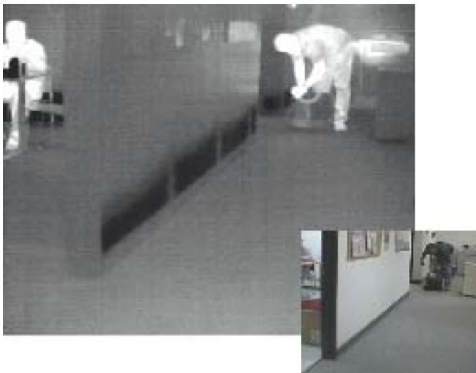
Figure 7. Incomplete Drying. Technicians pack up the drying equipment because it appears the floor is dry. But the thermal pattern suggests there is more moisture that must be removed to ensure that mold does not grow inside the wall.
