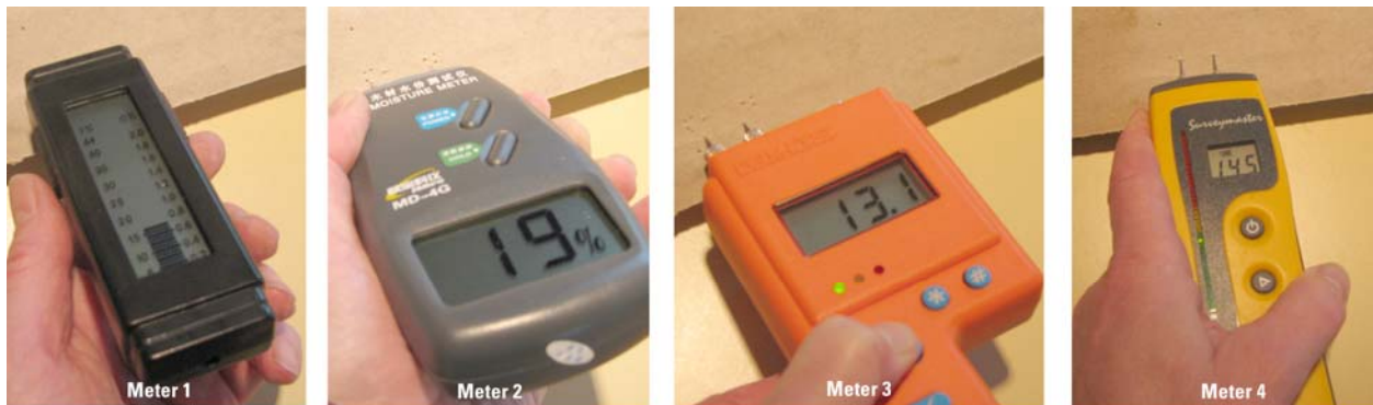
Figure 13. Meters from different manufacturers show different values for “saturated” moisture content.
