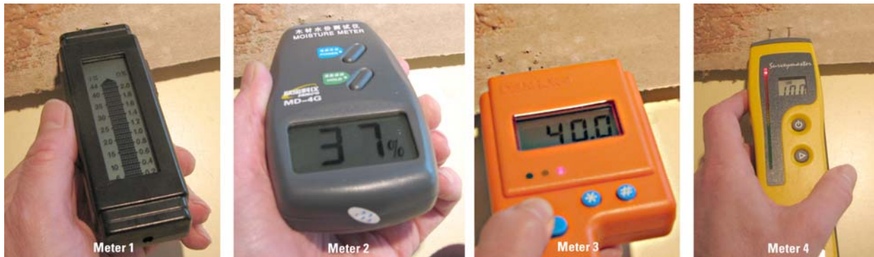
Figure 14. Different meters also show different values in the range of mold-risky moisture contents.
