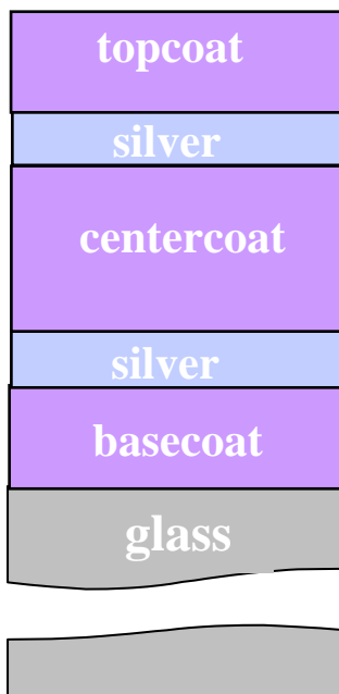
Figure 2. Schematic diagram of a double layer silver stack coatings with silver.
